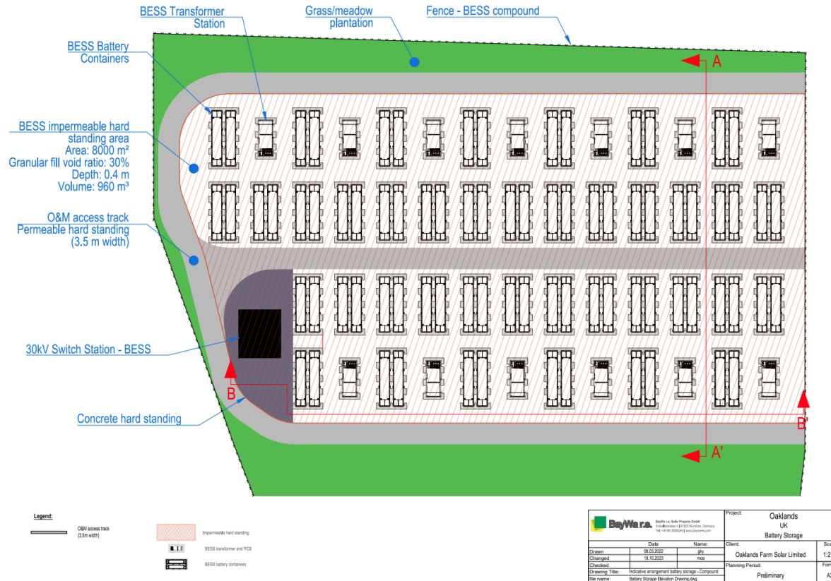
Figure 3: BESS Compound Layout
